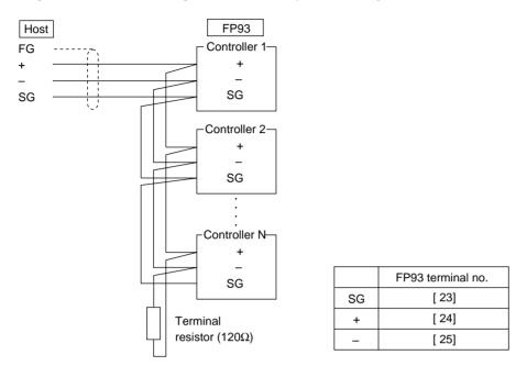
Note 1: In the case of RS-485, provide it with the attached terminal resistor of 1/2W, 120Ω across terminals + and if necessary. Nevertheless, it should be provided to only the last controller. If two or more controllers are provided with terminal resistors, correct operation cannot be guaranteed.
